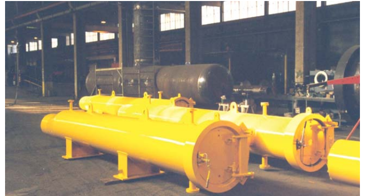
Figure 6: pipeline size 18" x 22" / 18" x 24" 300#
